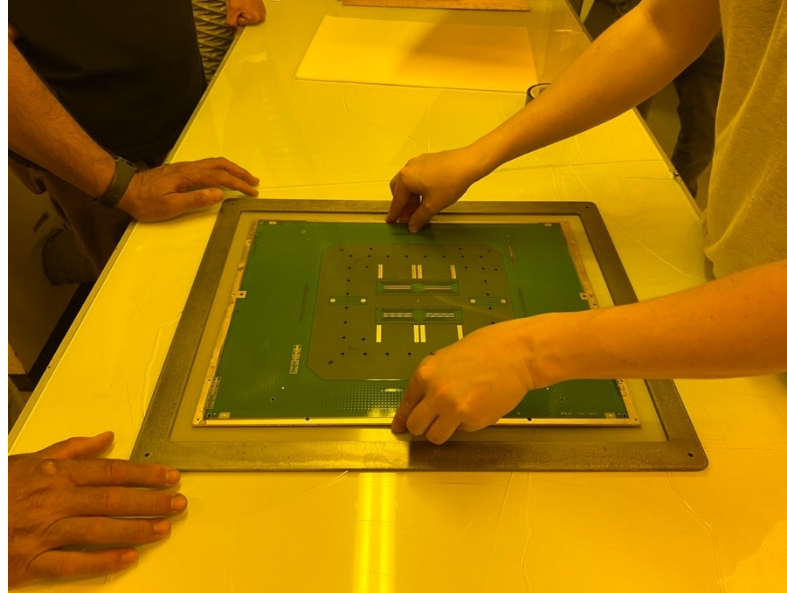
Laminated PCB positioned on the mesh before last (top) lamination
