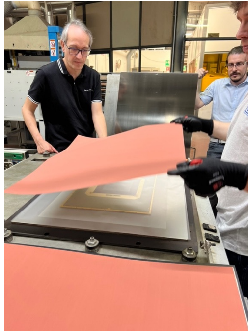
Pressing stack preparation with layers of: copper, conformable layer (pacoflex), soft layers, ...
