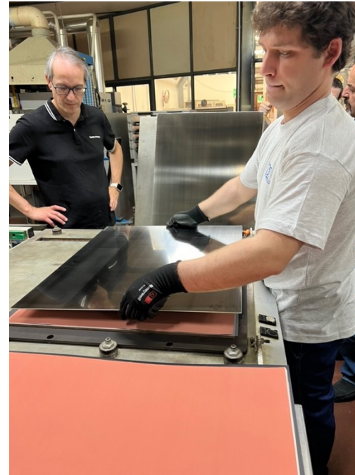
Pressing stack preparation with layers of: copper, conformable layer (pacoflex), soft layers, ...
