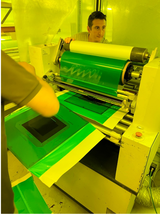
Laminated PCB positioned on the mesh before last (top) lamination
