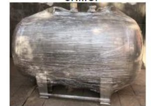
SF 6 storage tank
