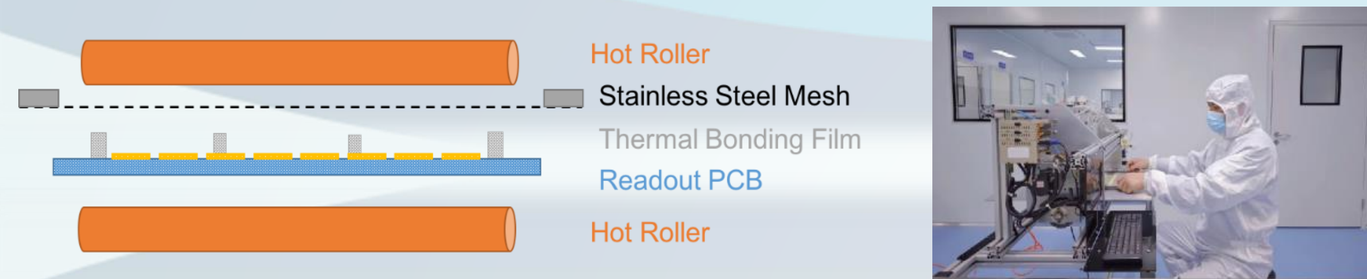
Fig. 1 the thermal bonding method of the Micromegas detector
