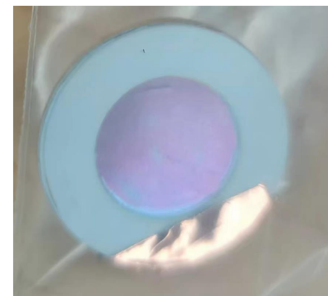
Figure.13 CsI plated on stainless steel mesh as a reflective photocathode
