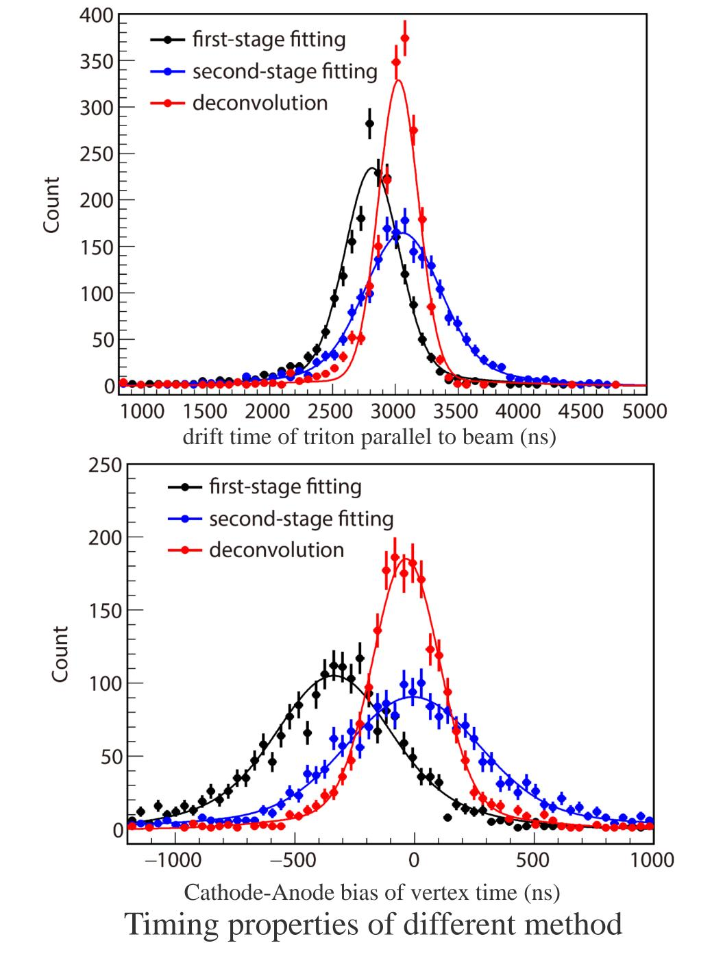
And signals are fitted via two steps: a full peak fitting (first stage fitting) and a rising edge fitting (second stage fitting).
