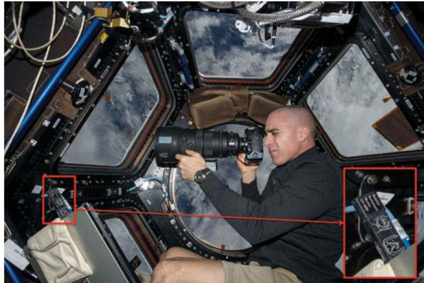
Astronaut Chrisey Cassidy in the ISS with a USB powered TPX particle tracker. The tracker for ISS has been completely developed at IEAP and delivered to NASA in 2012.
