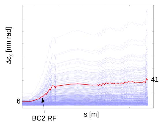
10% rms jitter, no ISR, with single bunch wakes, red line shows  $90^{th}$  percentile of single bunch emittances
