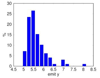
100 μm rms quads and bends, 50 μm rms sextupoles, 1 μm rms BPMs, 100 nm BPM resolution => p90 = 6.2 nm rad after DFS
