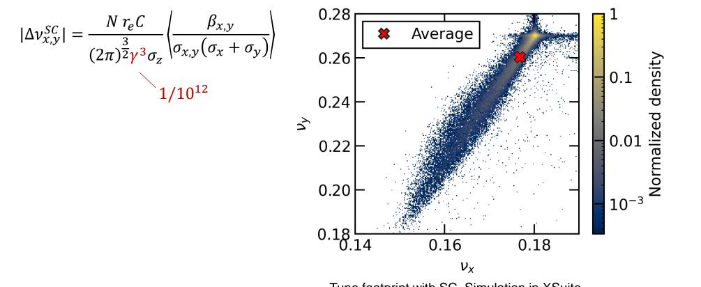
Tune footprint with SC. Simulation in XSuite. 10 nC bunch, 128 turns, long. wakes included, single-harmonic RF system
