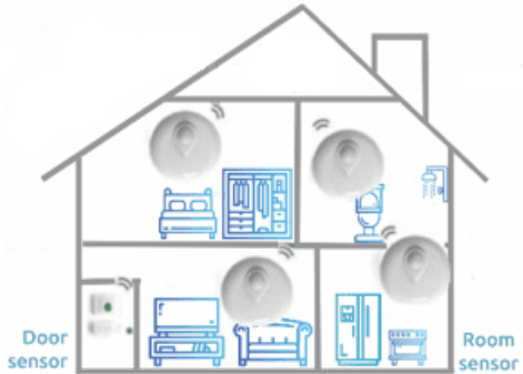
Motion sensors and magnetic contact sensor for presence monitoring and extracting ADL patterns
