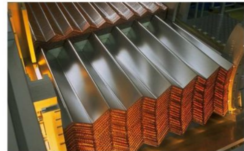
Picture of an electromagnetic end-cap module during stacking, showing the accordion structure of the ATLAS EM calorimeters.
