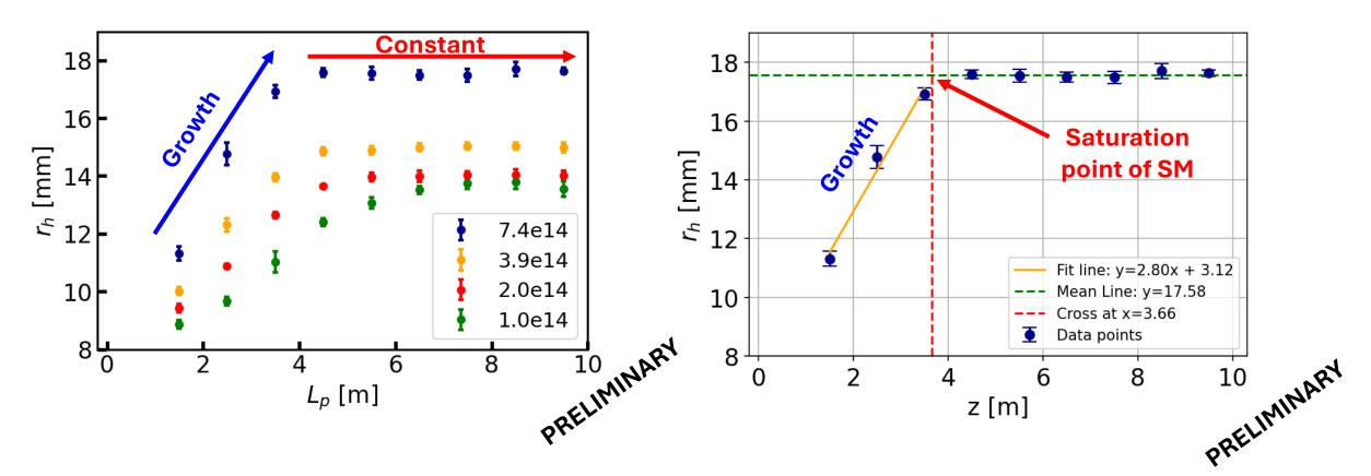
Repeat this measurement for **different plasma densities** We extract both the **saturation length** and the **"slope of the growth"**
