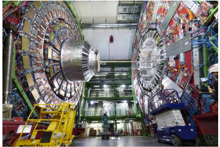
Figure 2 The CMS detector in the experimental cavern, one of four particle detectors for collisions in LHC accelerator.
