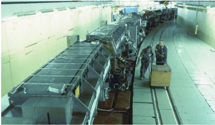
200-m diameter ring, weight of magnets 3,800 tons
