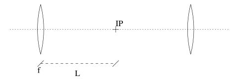
The beam enters the quadrupole with Twiss parameters  $\beta_0 = 20$  m and  $\alpha_0 = 0$ . The drift space has length L = 10 m.
