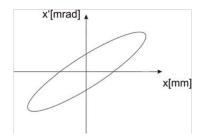
(III) when the beam is convergent. Answer. Convergent beam (negative slope):
