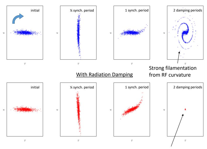
Injected beam dimensions reduce in both au and  $\epsilon$
