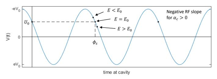
Particles which are high in energy travel further in single revolution and will arrive later Particles which are low in energy travel less distance and will arrive earlier
