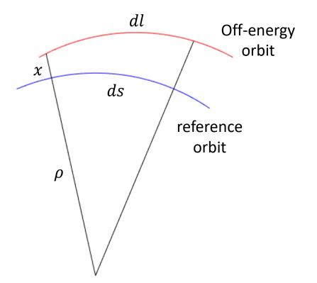
From the bend angle, the difference in path length between the on and off-momentum orbits is
