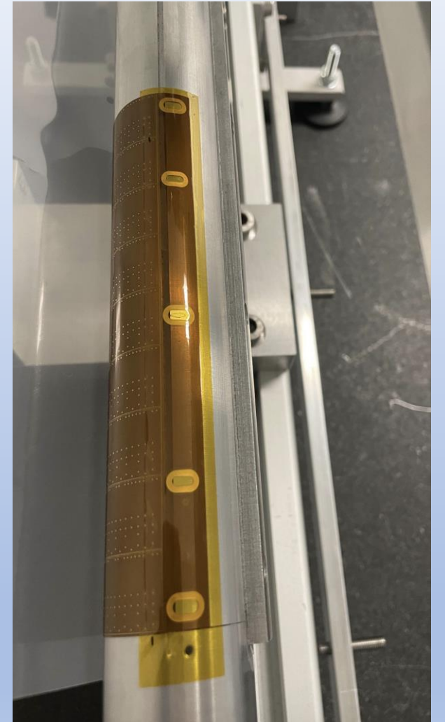
Bending test of ALPIDE wafer in IPHC
