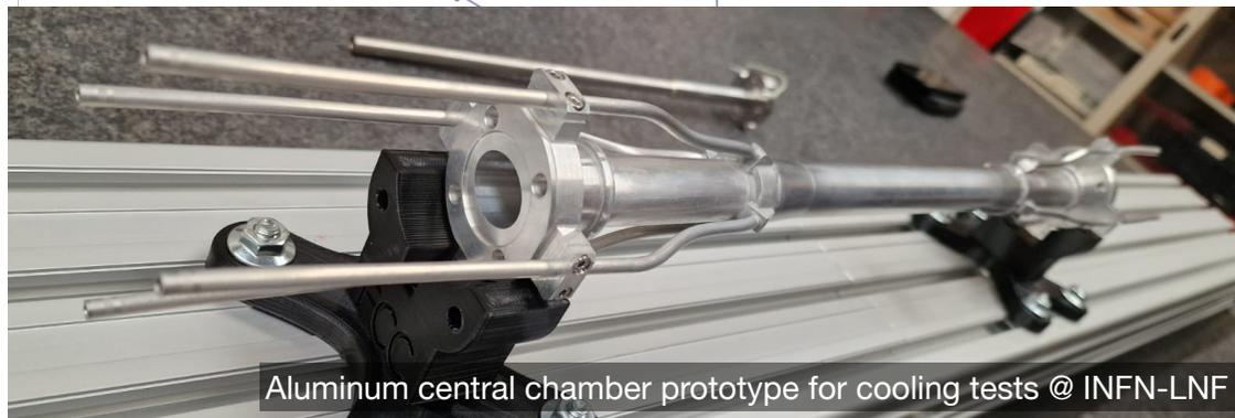
Aluminum central chamber prototype for cooling tests @ INFN-LNF
