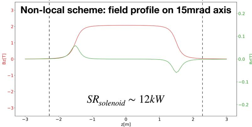
The **2T detector solenoids** induce coupling in the FCCee lattice.
