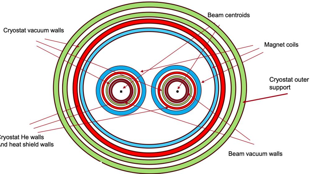
Proposal to have two **separate cryostats** for QC1 and QC2 on the same raft.
