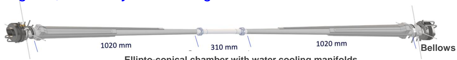
Ellipto-conical chamber with water cooling manifolds
