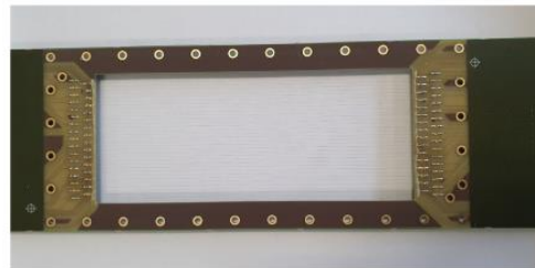
Carbon wire chamber soldered then glued
