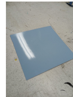
Thin melamine sheets ( \rho \sim 1.5 \times 10^{11} \Omega \text{ cm} ) and polycarbonate sheet to support the gas gaps
