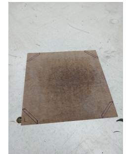
Thin melamine sheets ( \rho \sim 1.5 \times 10^{11} \Omega \text{ cm} ) and polycarbonate sheet to support the gas gaps
