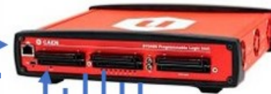
CAEN DT5495 Programmable Logic Unit
