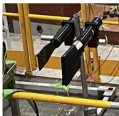
Scintillation counters Measure the beam intensity
