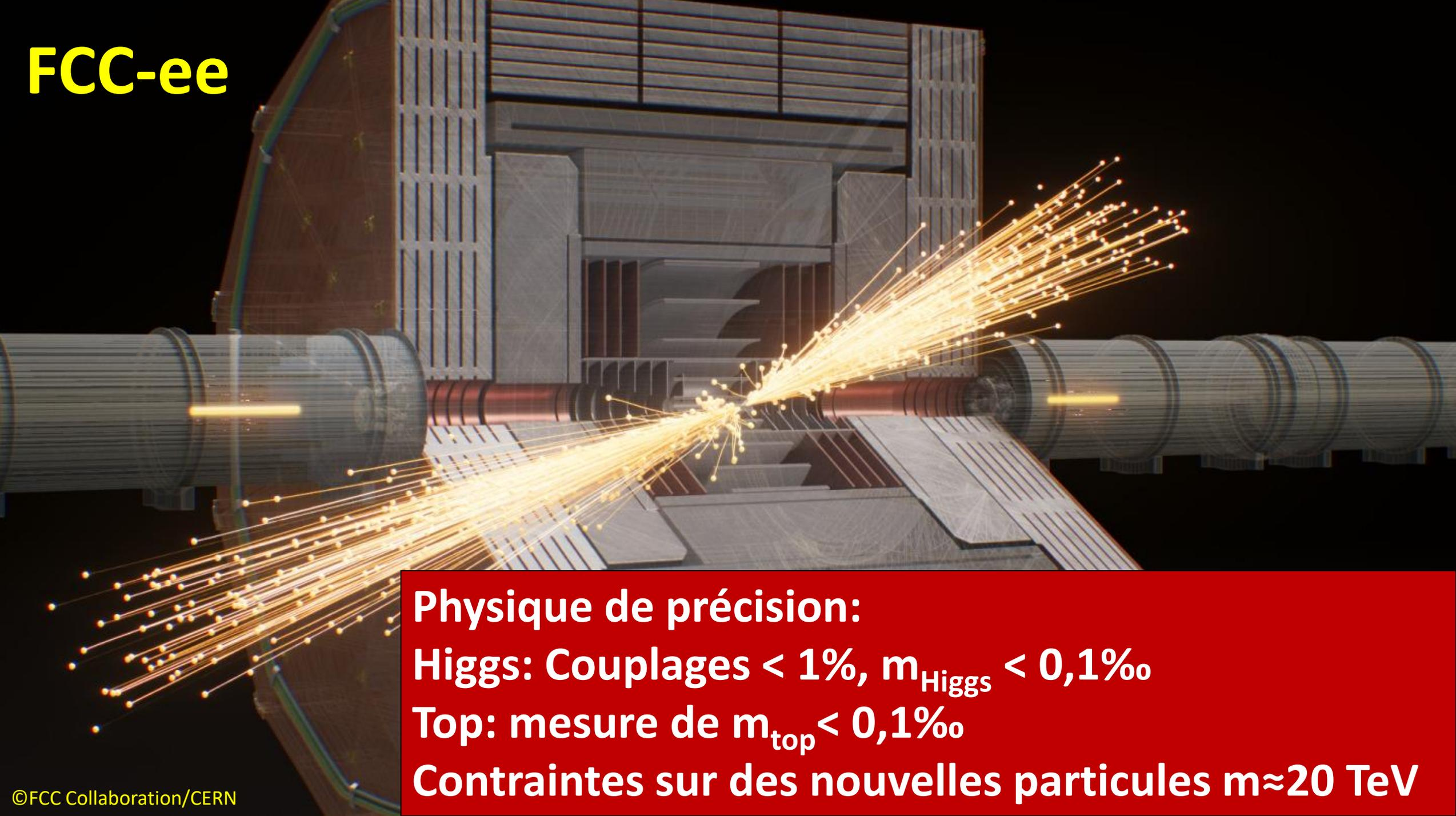
A 3D cutaway rendering of the FCC-ee electron-positron collider. Two large cylindrical beam pipes enter from the left and right, meeting at a central interaction point. At this point, a dense spray of golden-yellow particles is shown, representing the collision products. The surrounding structure consists of various metallic components, including magnets and shielding, all rendered in shades of grey and blue.
