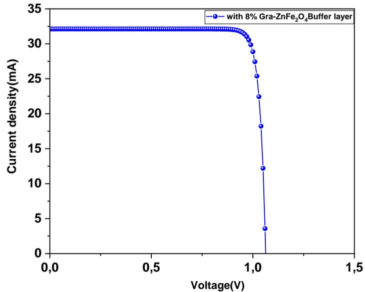
Figure: J-V Characteristic of the solar cell
