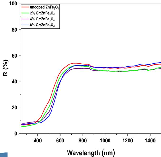
The undoped ZnFe<sub>2</sub>O<sub>4</sub> presents the highest reflectance, while the 4% Gra:ZnFe<sub>2</sub>O<sub>4</sub> showed the lowest reflectance.
