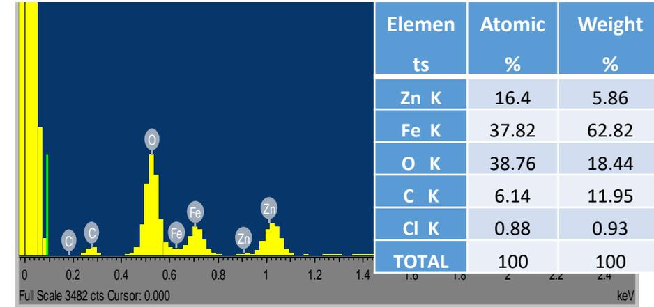
Figure : EDX analysis of 8% Gra: $\text{ZnFe}_2\text{O}_4$  thin films .
