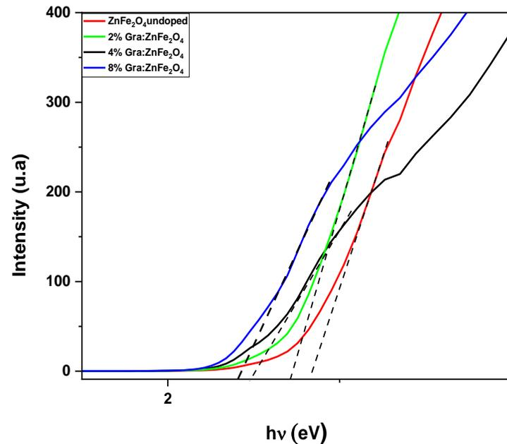
The Graphene doping contribute to the formation of intermediate energy levels within the band gap of zinc ferrite, facilitating electron transitions and reducing the overall band gap energy.
