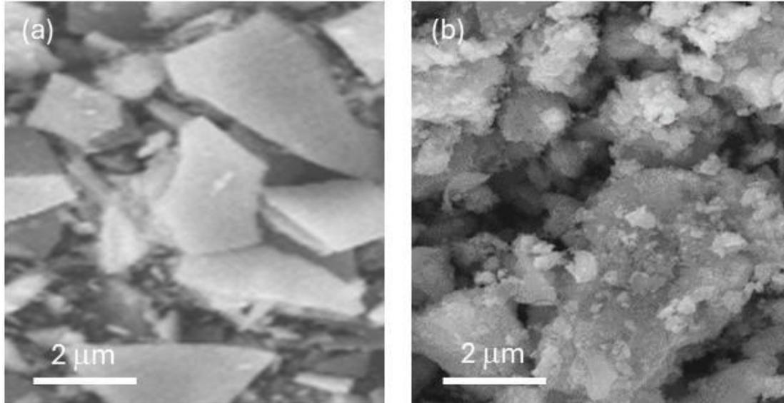
Figure : SEM images of a) undoped  $\text{ZnFe}_2\text{O}_4$  and b) Graphene 8% doped  $\text{ZnFe}_2\text{O}_4$  thin films .
