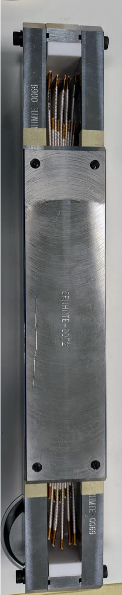
Open Impregnation Mould for HV 10-Stack
