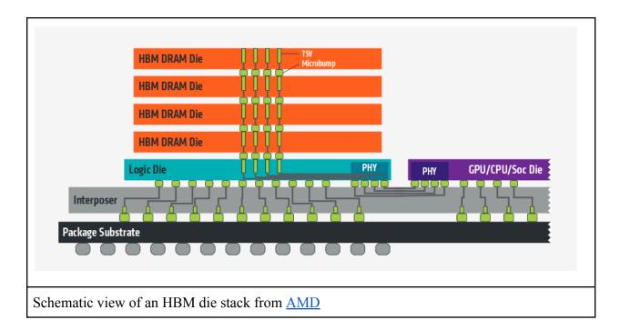
Although the "per pin" bit rate is low compared to GDDR5 (1 Gbps for HBM vs 10 Gbps for GDDR5), HBM achieves higher bandwidth by utilizing a 1024-bit wide interface per stack vs 32 bits per GDDR5 chip.
