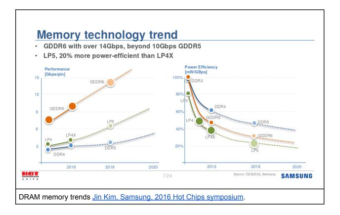
Since the introduction of the GDDR5 standard in 2008, JEDEC has been working on its successor, GDDR6. This new JEDEC standard was finalized in 2017. Memory capacity chip remains unchanged from GDDR5/5X at 8Gb. GDDR6 chips have been announced by Samsung and Micron in 2018 with data rates of up to 16 Gbps per pin.
