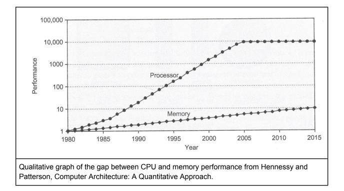
The impact of this growing gap in performance between memory and processor has been referred to as "<u>hitting the memory wall</u>". In order to mitigate the effects of hitting the wall, a computing system (CPU + memory subsystem) needs to be designed to compensate for this performance gap, or the application (software) needs to be re-written with algorithms and coding
