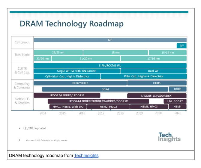
The development of DRAM fabrication faces several challenges in further shrinking the structure sizes, which explains the lag in DRAM nodes with respect to logic nodes. Below a certain threshold in feature sizes, electrical resistivity increases nonlinearly, requiring new materials and new capacitor shapes to be evaluated. Similarly, crosstalk between cells becomes an issue, which can be mitigated by using new types of dielectrics. Lithography patterning and exposure
