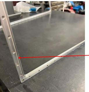
Oring groove 2 mm wide 1.7 mm deep for 2 mm orings
