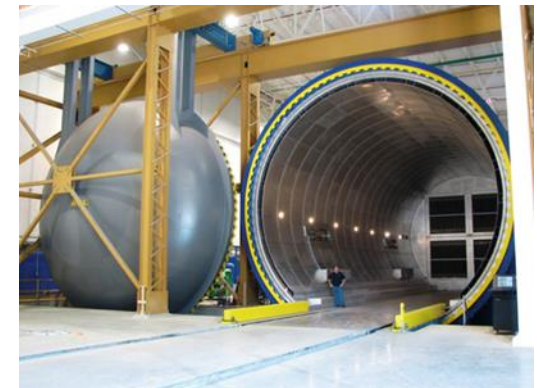
A large autoclave that is used to make the wings of Boeing 787
