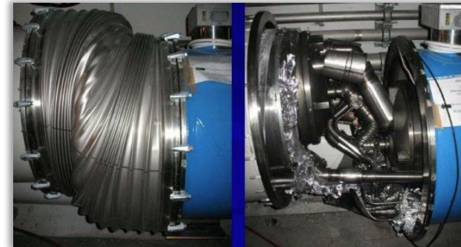
Damaged LHC dipole interconnexion
