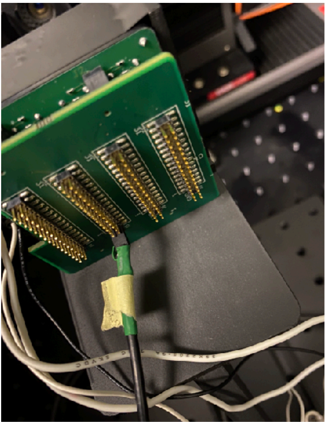
Backplane adapter board (using GSI PCB design from A. Lehman et al.)
