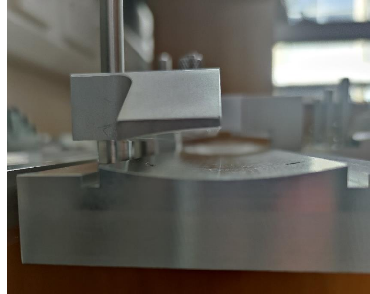
Vacuum Chuck on Module Installation Tooling
