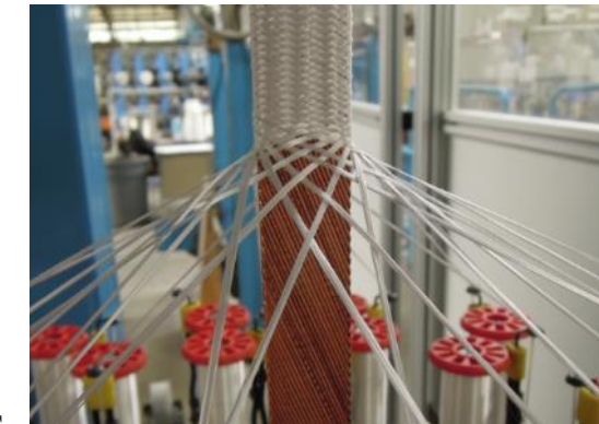
Nb 3 Sn (Precursor) Cable Insulation being Braided
