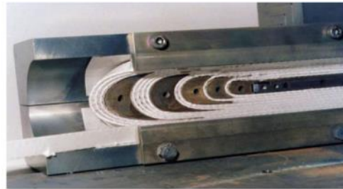
Fig. 4.12 End view of a reacted coil inner layer. (Courtesy of ELIN, Austria)
