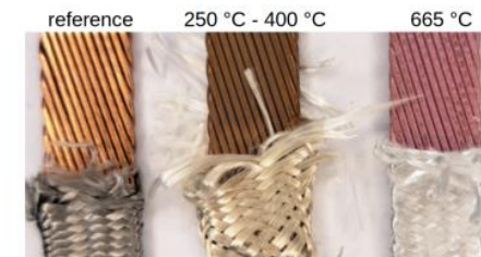
Fig. 4. Images of Rutherford cables after the RHT, with and without the introduction of oxygen.
