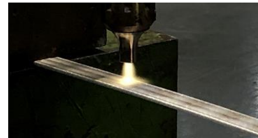
Example Plasma Treatment on a Nb 3 Sn Cable
