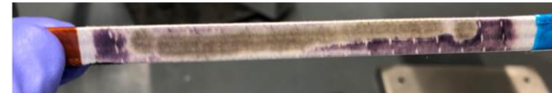
Iodine Test after Plasma Desizing of S2 Glass (636). 1mm Distance, 1.5m/s Moving Nozzle
