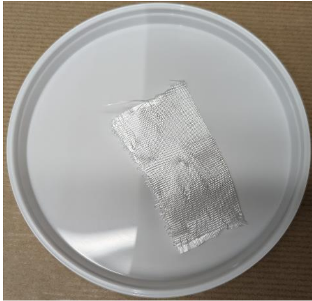
Appearance following Thermal Desizing
