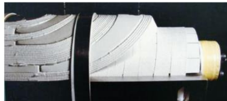
Fig. 6.9 Layer 2 return end before reaction (end spacers coated)
