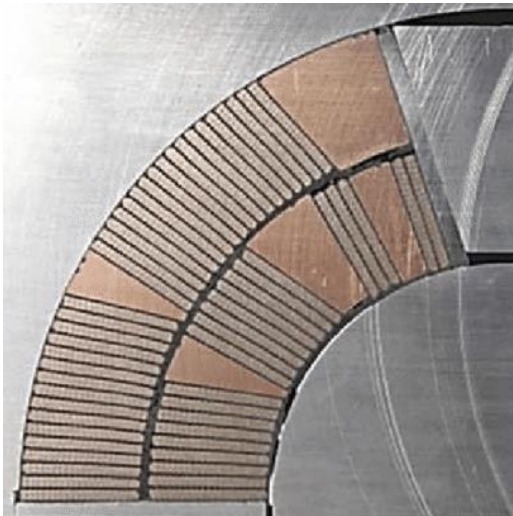
Section of a Nb_3Sn dipole magnet
