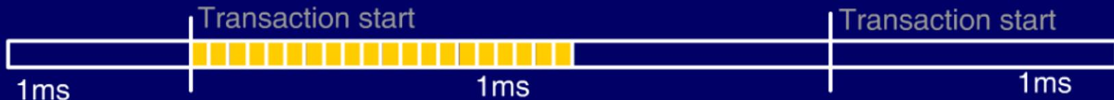
→ Unless protocol uses transactions comprised of a multiple of 24.576 (that's 24 point...) packets, the nominal bandwidth cannot be achieved. And even then...
