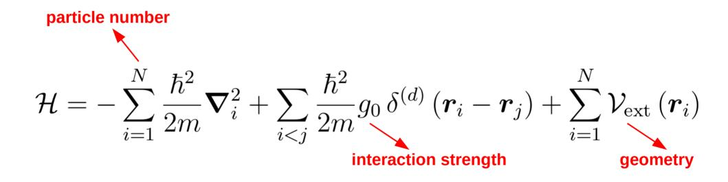
Parameters can be tuned in a table-top experiment
