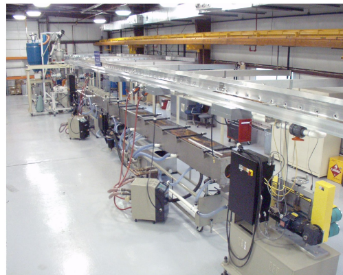
Figure 14. The scintillator extrusion facility at Fermilab.
