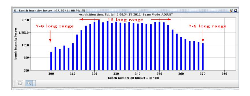
Losses of the bunches in a batch
