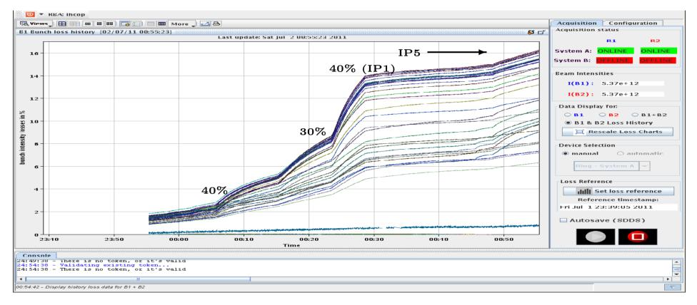
→ Loss as function of crossing angle (IP1 and IP5)
