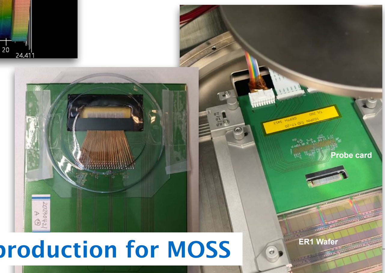
FPCB for APTS-SF design and production APTS-SF Carrier board modification
