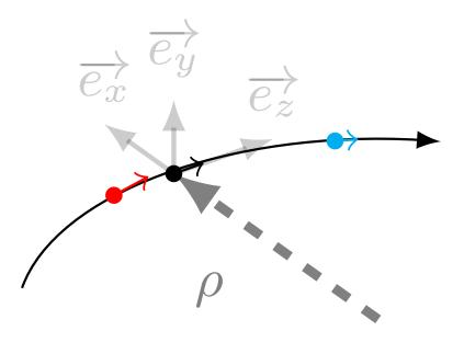
• The acceleration is done by applying an electric field tangential to the beam trajectory with
