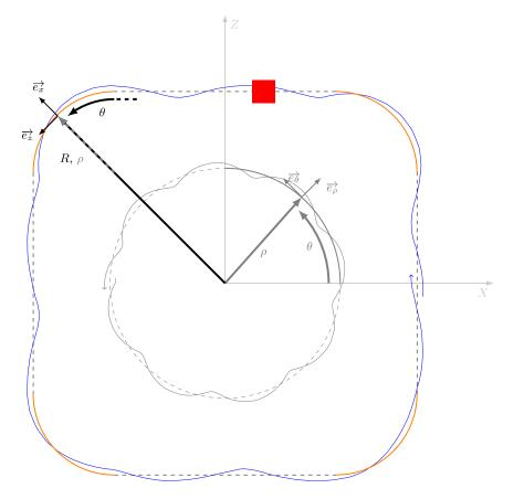
ullet It is also important to disembiguate ho which is the bending radius and R which is the particle orbit including straight sections of total length L. We have
