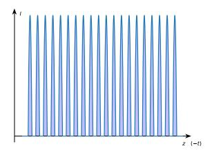
Depending on the destination (experiment or next machine in a chain), parameters defining the synchrotron motion can be adjusted to deliver a continuous or bunched beam.
