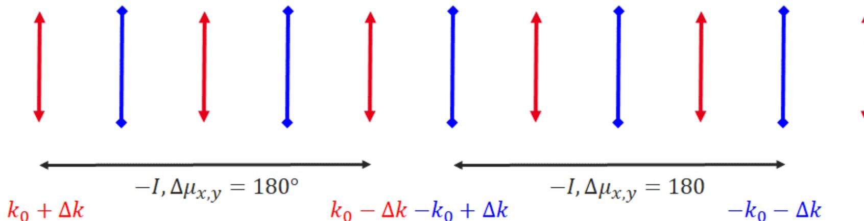
$$\Delta k \approx \frac{\sqrt{x}}{2\sqrt{3}} \text{ with } x = \frac{\alpha}{\alpha_0} - 1 \text{ where } \alpha \text{ is the momentum compaction and } 0 \text{ when } \Delta k=0$$
