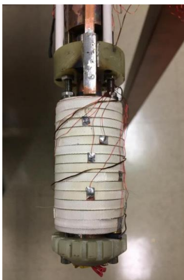
Figure 9: HTS solenoid (non-insulated) generating 14.4 T in the bore of a 31.1 resistive background, reaching record fields of 45.5 T [Nature 570, 496-499, 2019].
