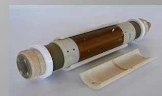
Rotating coils with various diameters, lengths, and coil arrangement
