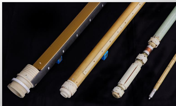
Rotating coils with various diameters, lengths, and coil arrangement
