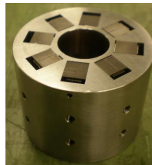
LINAC4 DTL PMQ, < 1 kg
