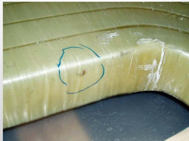
Poor penetration or wetting can lead to defects during operation
