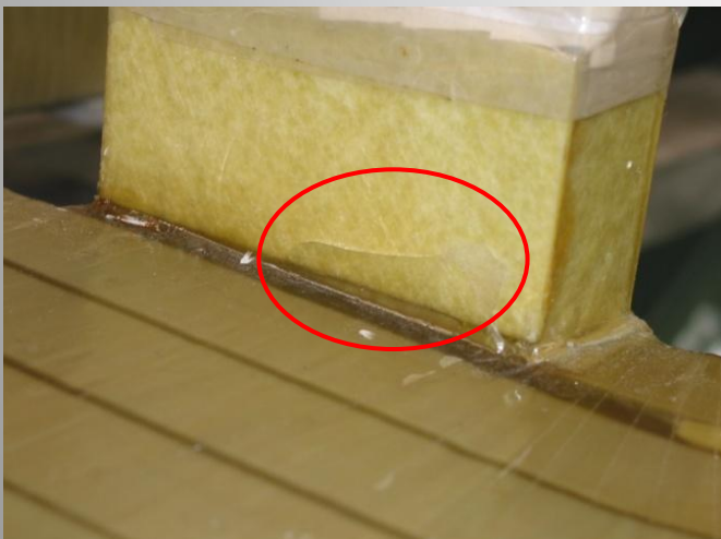
Obvious defects, like lack of resin bubbles, voids, fissures, cracks
