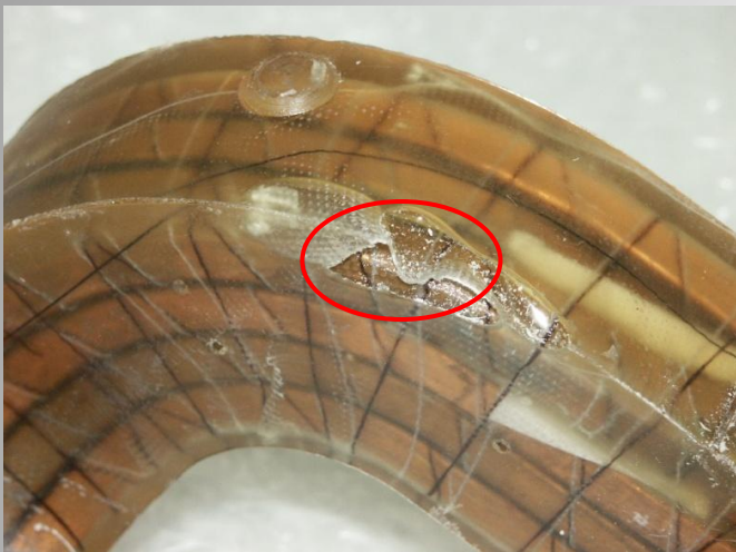
Obvious defects, like lack of resin bubbles, voids, fissures, cracks
