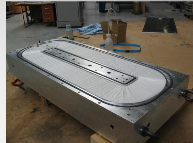
Vacuum impregnation with epoxy resin in auto-clave or vacuum mold
