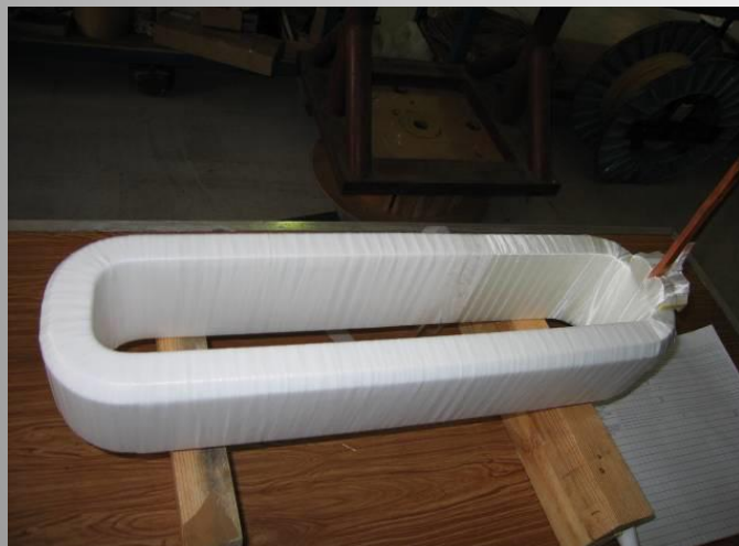
Interturn and mass insulation by several layers of glass-fibre tape
