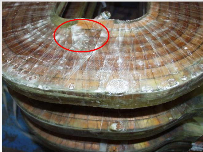
Poor penetration or wetting can lead to defects during operation
