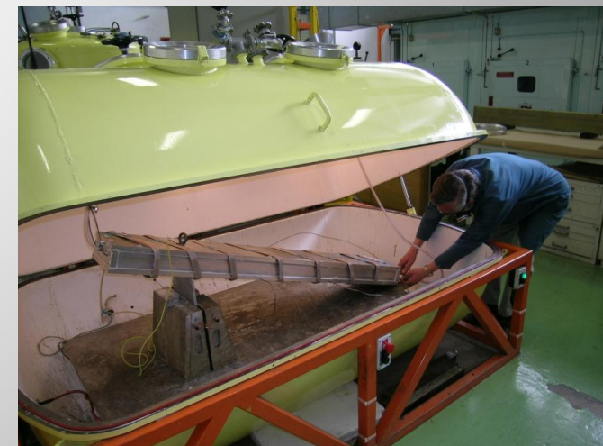
Vacuum impregnation with epoxy resin in auto-clave or vacuum mold
