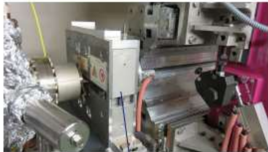
ESRF canting magnet (dipole field)
