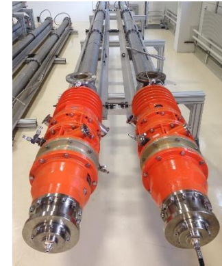
Picture: Coaxial loads for the SPS 200 MHz cavity © CERN
