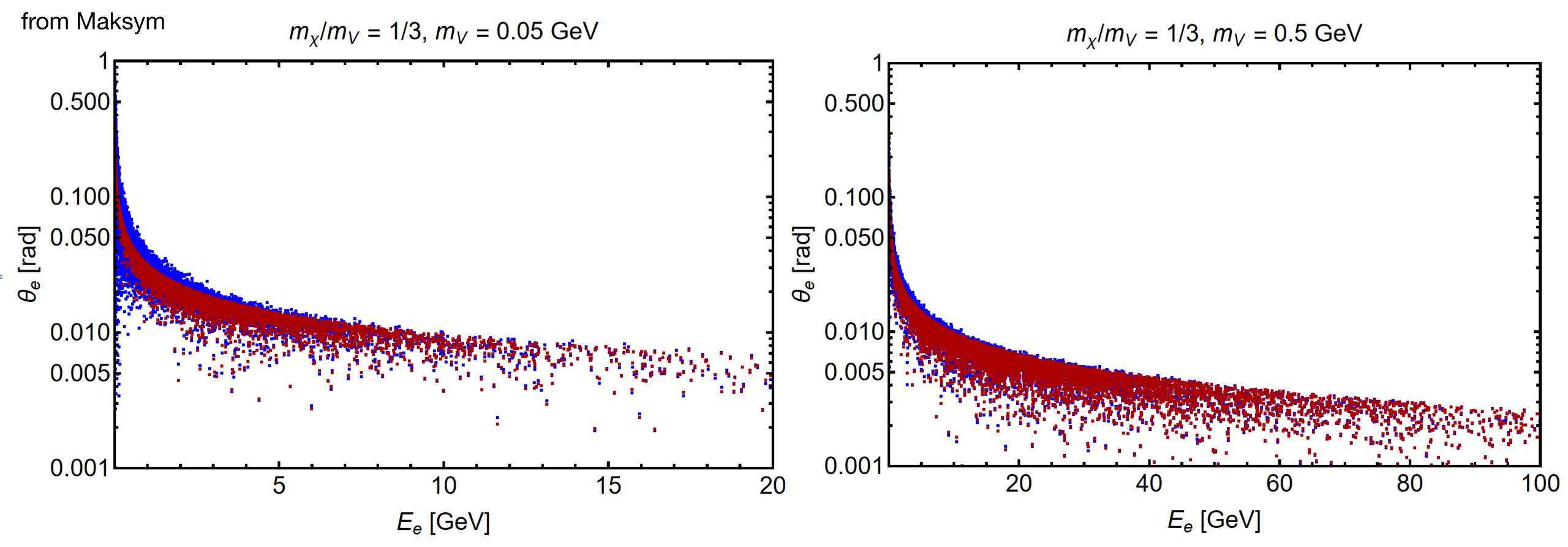
The plot shows the distribution of the recoil electron's energy ( $E_{p}$ ) versus its angle ( $\theta_{p}$ ) relative to the incoming  $\chi$ .  $m_{\chi} = m_{\chi} = m$
