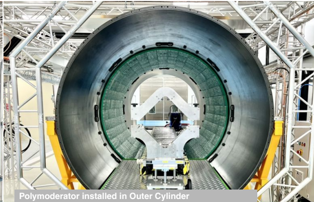
Polymoderator installed in Outer Cylinder
