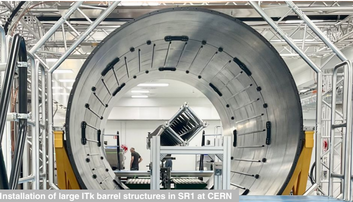
Installation of large ITk barrel structures in SR1 at CERN
