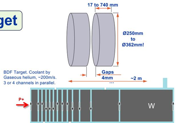
BDF Target. Coolant by Gaseous helium, ~200m/s. 3 or 4 channels in parallel.
