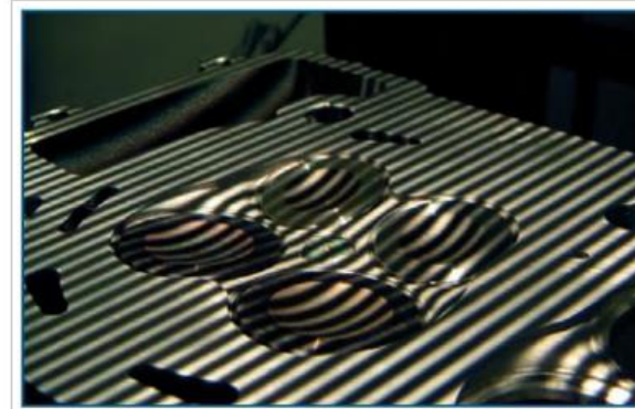
Acquisition of a motor combustion chamber by fringe (stripe) projection; analysis of the three-dimensional dataset (measuring area 100 x 100 mm)
